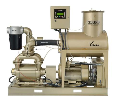
The outer shell acts as a condenser, as the surrounding ambient air is cooler than the discharge stream, allowing a condensing effect of the seal fluid from the air stream.
