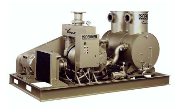
Operating principles are very similar to that of the standard Vmax systems. Seal fluid flows from the separator tank, through the heat exchanger to the vacuum pump. The large capacity vacuum pump produces vacuum as described in the <a href="Principles of Operation">Principles of Operation</a>— Single Stage Liquid Ring Vacuum Pump. The seal-fluid separation process through the reservoir tank also remains similar to the standard Vmax systems.
