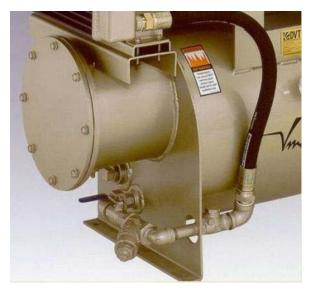
The seal fluid enters the heat exchanger through the lower seal-fluid line. Seal fluid exits the heat exchanger and feeds the pump. The seal fluid is pushed by tank pressure and pulled by a vacuum created by the pump.
