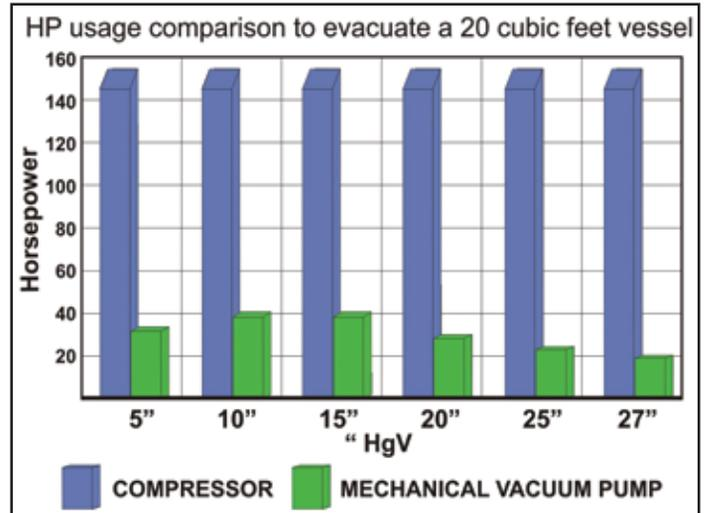
Industry can save thousands of dollars by shutting down an air compressor and switching to mechanical vacuum pumps.
