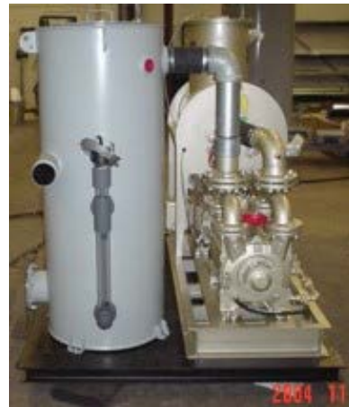
Dekker Vmax System with knock-out tank.
