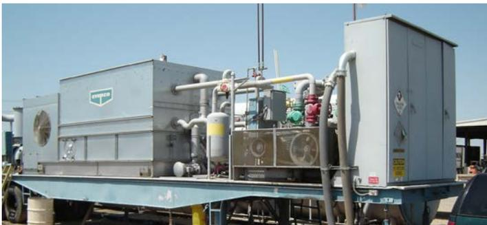
Vacuum pump and condenser unit on flatbed
