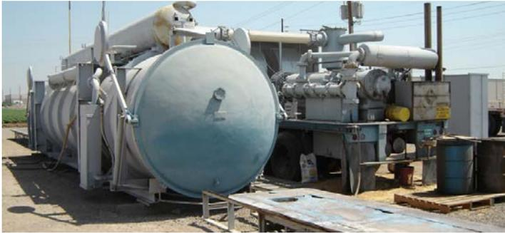
Vacuum cooling chamber on skid
