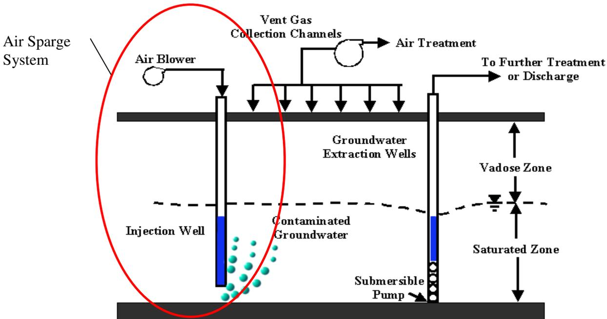
Figure 2: Simplified illustration of an air sparge system used in combination with a multi-phase extraction system
