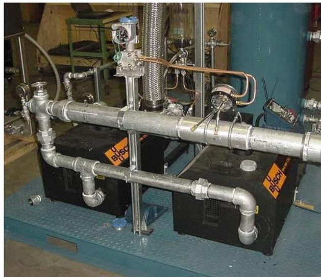
Figure 7: Dual rotary claw compressor package
