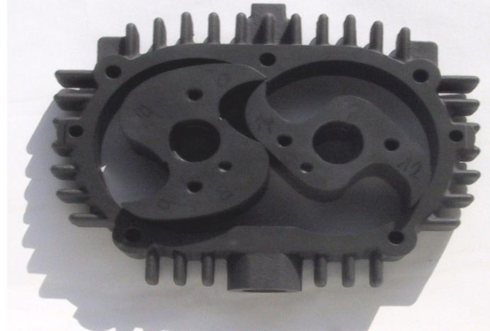
Figure 8: Internal workings of a rotary claw compressor
