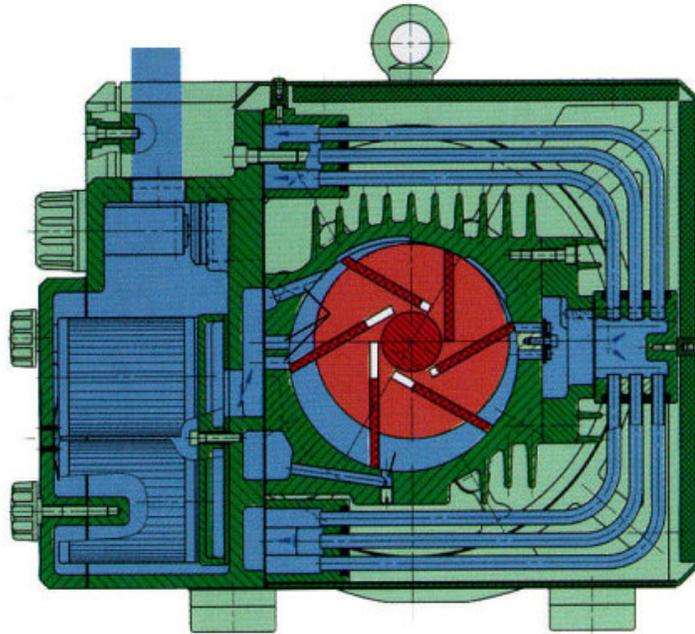
Figure 6: Internal working of a rotary vane compressor
