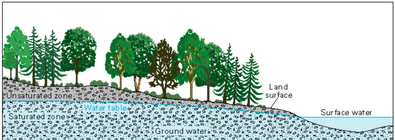
Figure 1: Illustration of groundwater table and the saturated and unsaturated zones of soil
