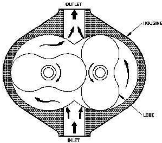
Figure 4: Internal working of a rotary lobe compressor
