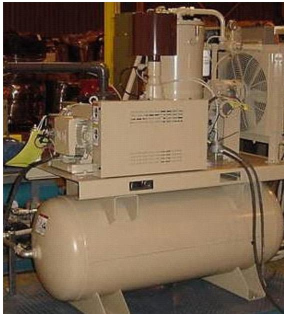
Figure 9: Rotary Screw Compressor Package
