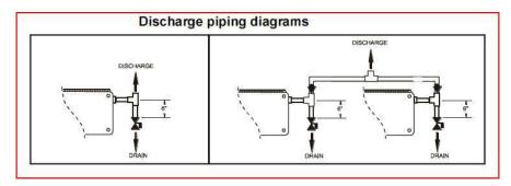
Refer to the Installation, Operations, and Maintenance Manual for more information on proper discharge piping.
