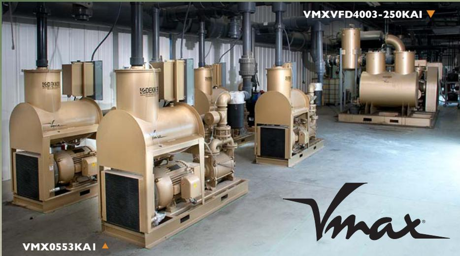
Liquid ring vacuum pumps are widely employed in demanding industries like plastics processing for CNC hold-down because of their high tolerance of liquid and solid carryover without compromising the pumps' mechanical integrity or efficiency. Unlike other types of vacuum pumps, liquid ring machines don't need to be rebuilt or replaced on a regular basis. The pump has only one moving part, and there is no metal-to-metal contact between the components and the casing, making the pump wear-free.
