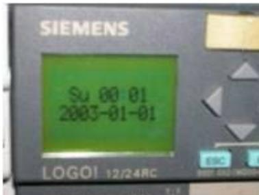
From the Date/Time screen, open the Menu screen by pressing the ESC button.
