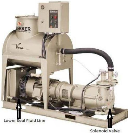
From the heat exchanger, the seal fluid flows through the lower seal-fluid line to the solenoid valve then to the vacuum pump. The static head from the overhead-mounted reservoir, together with the vacuum in the pump, pulls the seal fluid through the heat exchanger.
