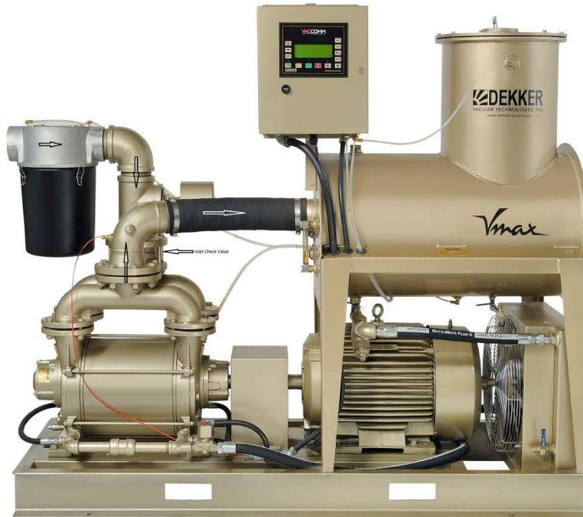
The outer shell acts as a condenser, as the surrounding ambient air is cooler than the discharge stream, allowing a condensing effect of the seal fluid from the air stream.
