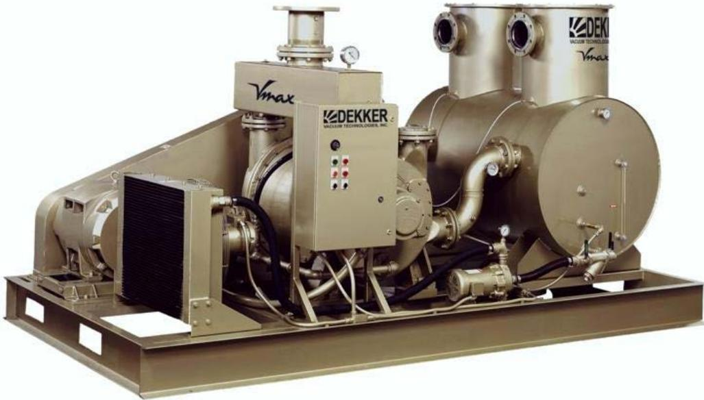
Operating principles are very similar to that of the standard Vmax systems. Seal fluid flows from the separator tank, through the heat exchanger to the vacuum pump. The large capacity vacuum pump produces vacuum as described in the [Principles of Operation — Single Stage Liquid Ring Vacuum Pump](#). The seal-fluid separation process through the reservoir tank also remains similar to the standard Vmax systems.
