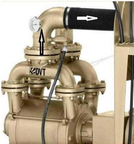
Discharged seal fluid, together with process gas, exits the discharge manifold, past the temperature switch and temperature gauge, back into the separator tank.
