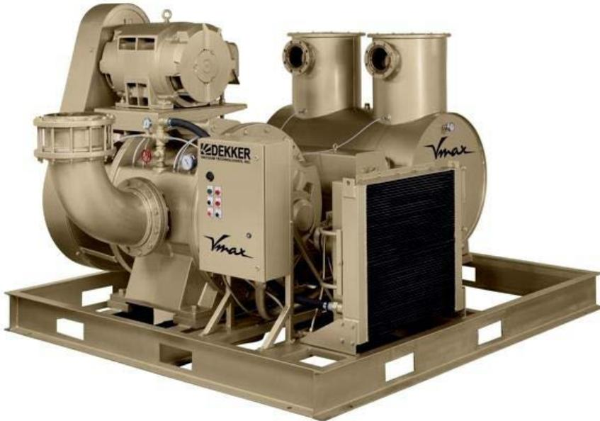
Seal-fluid flow is regulated by a globe valve and compound gauge located between the circulation pump and the vacuum pump. Compound gauge pressure is usually regulated to 0 psig. Excessive pressure indicates too much seal fluid to the vacuum pump. Excessive vacuum indicates too little seal fluid to the vacuum pump.
